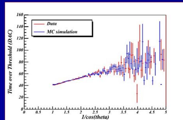
Fig. 8. ToTs vs  $1/\cos\theta$  and MC comparison
