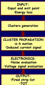
Fig. 3 Block diagram of SSD simulation code
