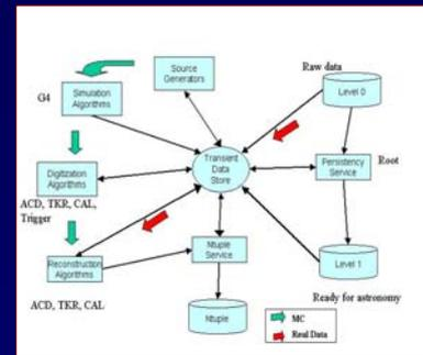
Fig.2 GLAST simulation/reconstruction data flow
