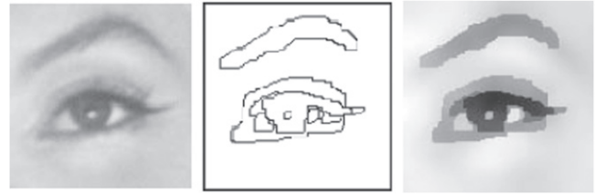
Figure 5. Left: image of an eye ( g ). Center: contours of the image in the Mumford–Shah model (edges \Gamma ). Right: piecewise smooth function approximating the image (cartoon u ) [32].
