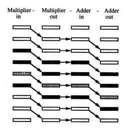
Not providing separate add and multiply instructions actually *improves* the processor efficiency, as it helps filling the pipeline.
